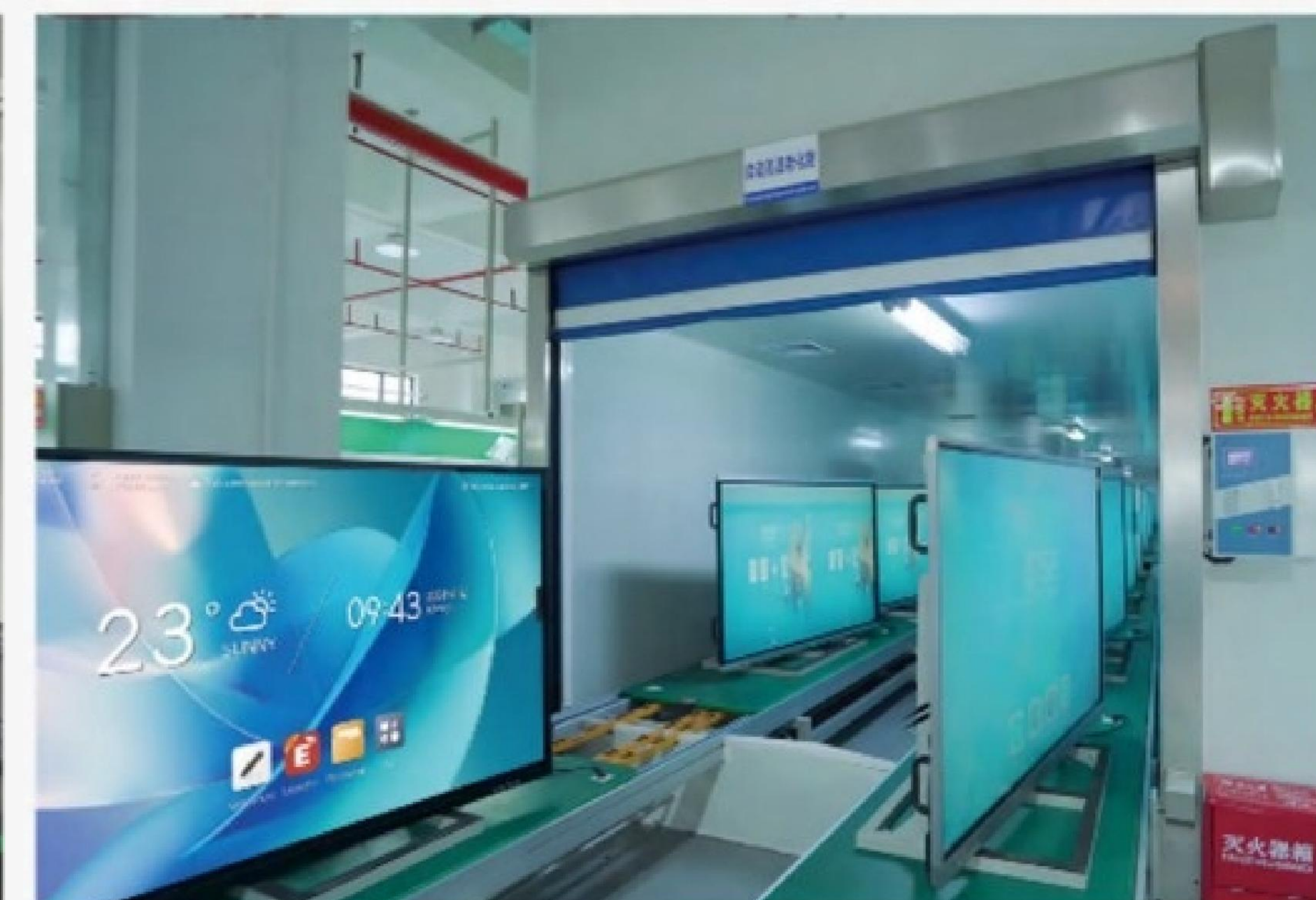
Fully automatic high temperature aging workshop
